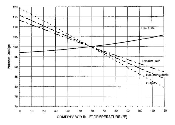
Figure 5 Typical Generator Performance Graph Provided by Manufacturers
