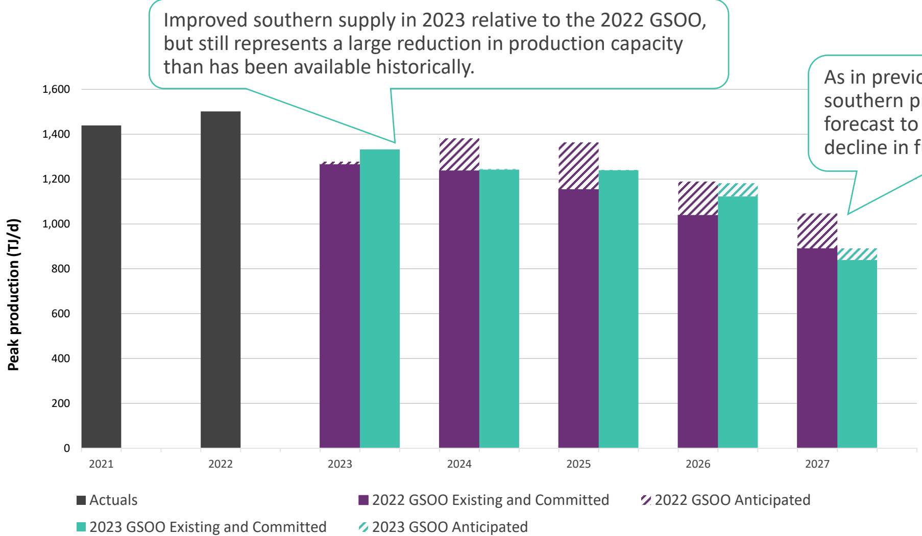
Figure 3 Actual and forecast maximum daily production capacity from southern gas fields, 2021-27 (TJ/d)
