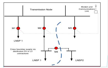
*Transmission network connection point(s)* feeding different LNSP areas. The above configuration illustrates:
