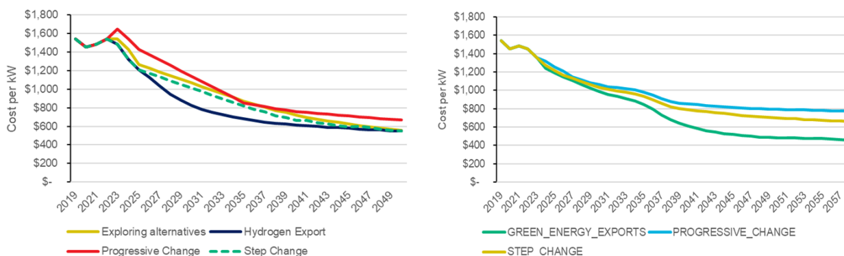
Figure 4 GEM view on fully installed residential PV system costs 2023 IASR (left), Draft 2024 FAU (right)
