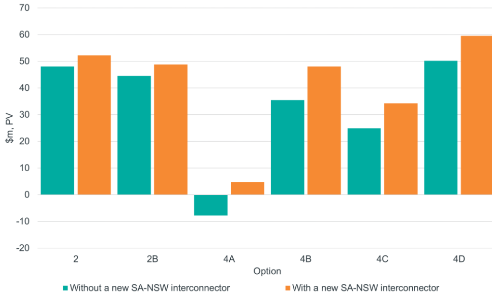
Figure E.5 – Summary of estimated net market benefits for credible options going via Yadnarie 13 assessed under the ‘core’ 14 set of assumptions
