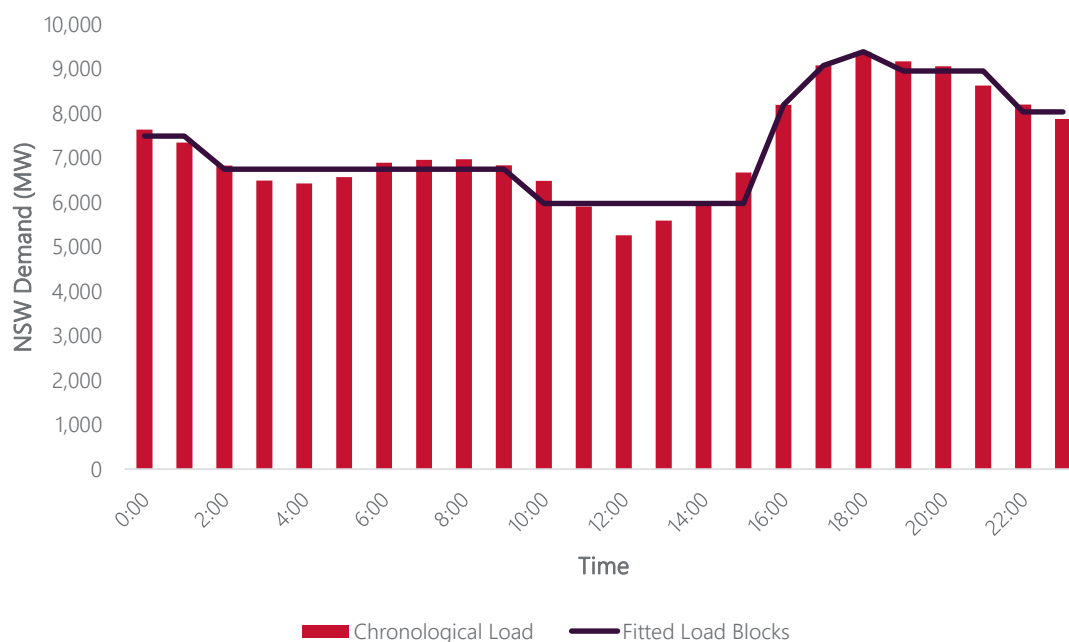
Figure 22 Example representation of fitted load blocks
