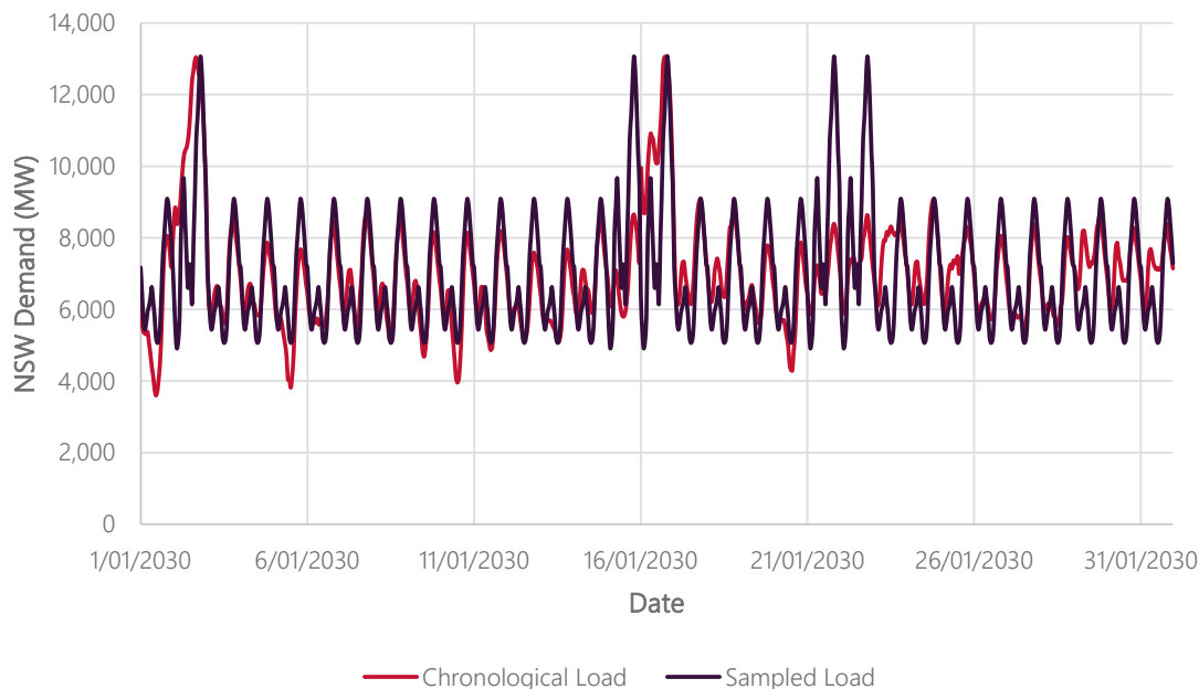
Figure 21 Example representation of a sampled load profile
